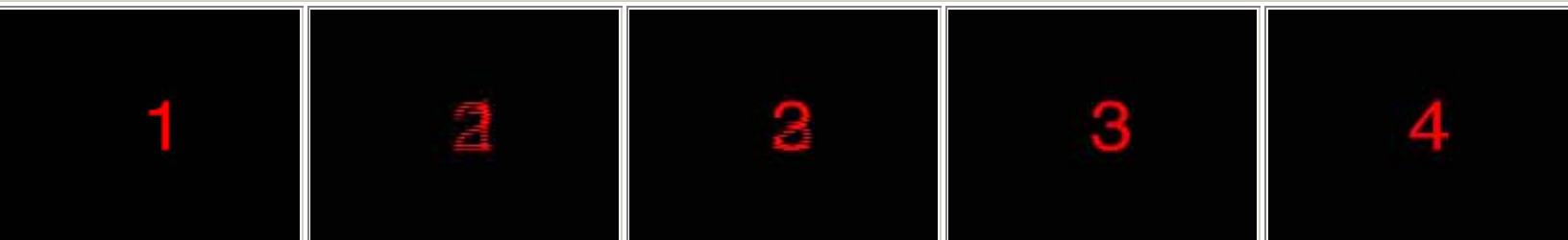
5 Output frames at 30fps, converted from 24fps using 3:2 pulldown
